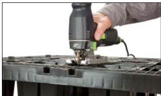
Separation of a basic element along the cutting mark
